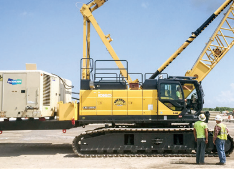
A custom power pack frame designed in-house for Kobelco pile driving cranes, approved by the manufacturer to match the structural and tipping capacities of the cranes.
